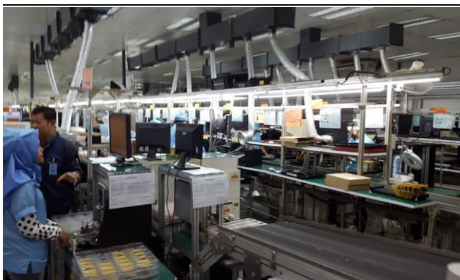
Figure 4: Printed Circuit Board (PCB) manufacturing line
